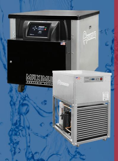
Advantage's Maximum Series Portable Chillers are refrigeration units coupled with an integral fluid circulation system that range in cooling capacity from 1/4 to 40 tons. These units are used to cool fluids to support industrial process cooling applications requiring a fluid temperature range from 20°F to 80°F.
